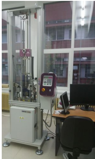
Fig. 3. Drop tower INSTRON Ceast 9340.
