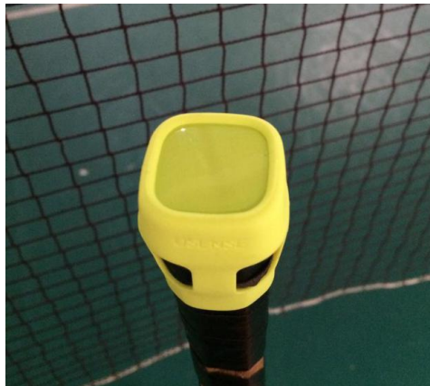
Fig. 3 The installation site of the three-axis acceleration sensor on the racket
