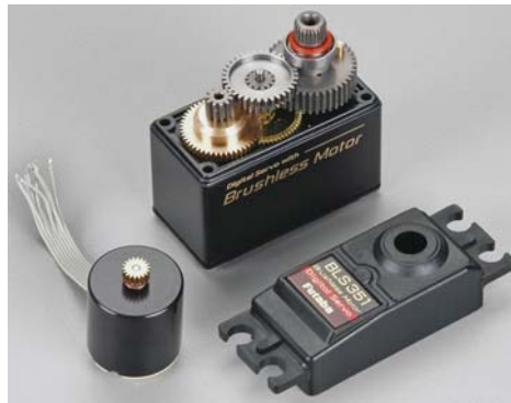
Fig.5. The elements of a Futaba servomotor
