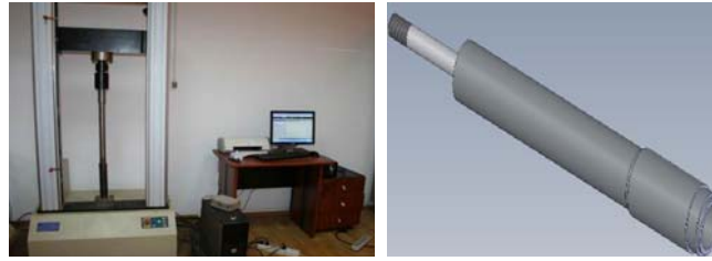
Fig. 1. Force machine used in the process of compacting biomass
