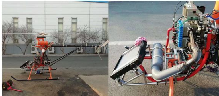
Fig. 8. Customized structural design of unmanned aerial helicopter
