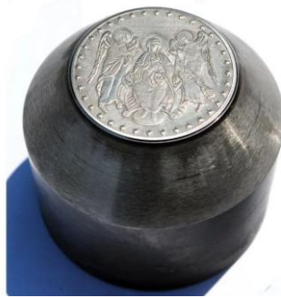
Fig. 2. A component of die (the positive mold with which the other molds are made)
