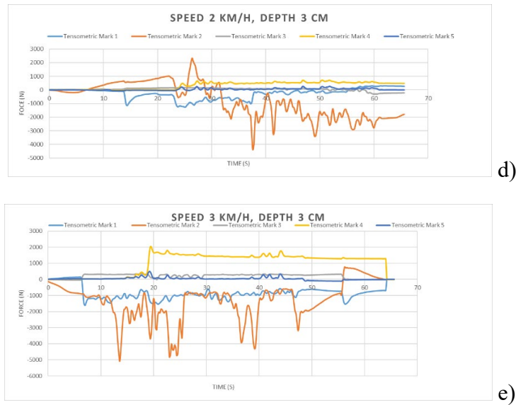
Fig.4. Graphs of forces measured using strain gauges a) speed 1 km/h, depth 1 cm, b) speed 2 km/h, depth 1 cm, c) speed 3 km/h, depth 1 cm, d) speed 3 km/h, depth 3 cm, e) speed 3 km/h, depth 3 cm.
