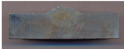
Fig. 4: Cross section of a API X65 plate after welding.
