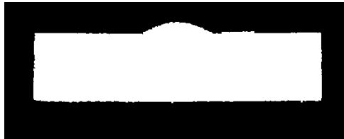
Fig. 8. separating the plate's cross section from image background.
