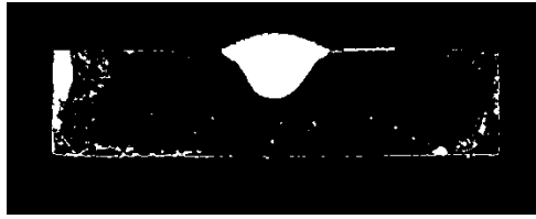
Fig.9. Separation of weld metal from other regions of image.
