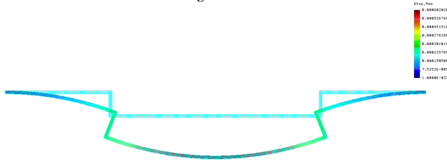
Fig.15 Z-shaped thermal microactuator after simulation
