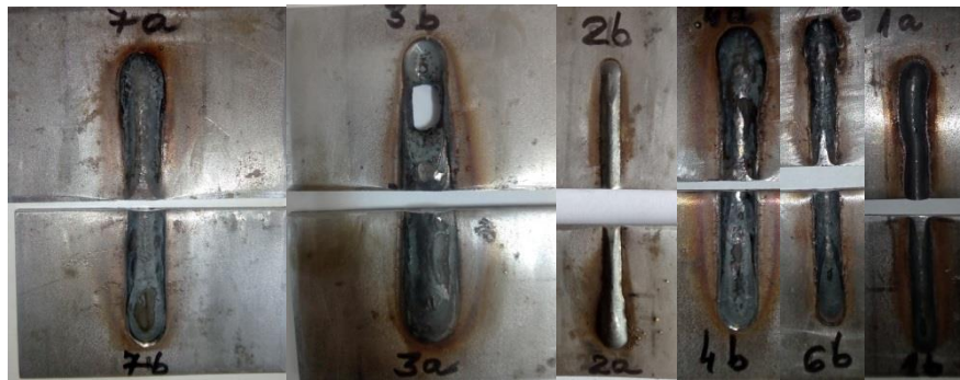
Fig. 4. Samples cut to prepare metallographic samples
