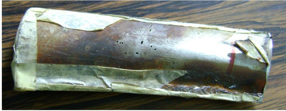
Fig. 1. Heat transferring unit section exposed to corrosive process
