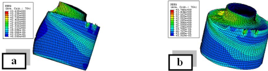
Fig. 9. Strain distribution pattern; (a): in the middle of process, (b): at the end of process (Billet diameter = 36 mm, Eccentricity = 6 mm)
