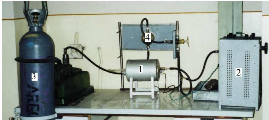
Fig. 1. Horizontal furnace for determinations on coke
