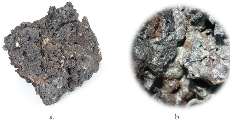
Fig. 6. Experimental agglomerate: a) by-product and b) stereo-microscope image
