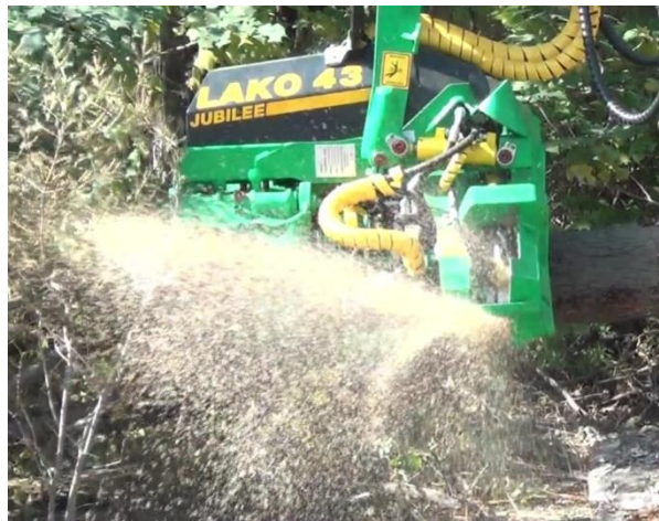
Fig.2 Timber cutting operation of the harvester head
