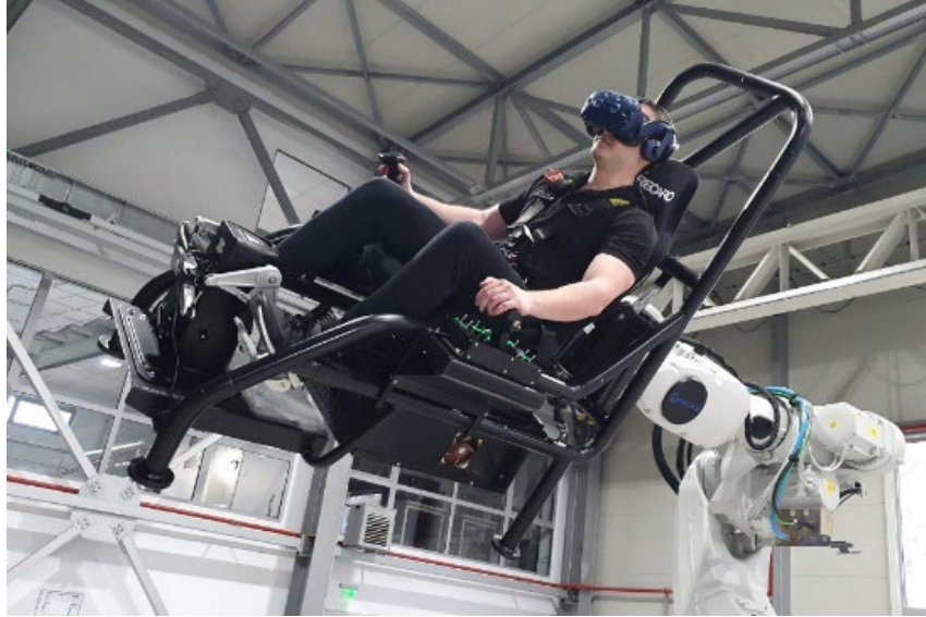
Fig. 1 Dynamic simulation system for pilot-in-the-loop applications – 6DoF flight simulator RoFSim
