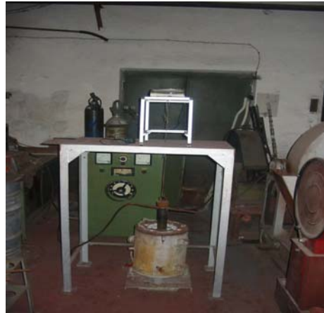
Fig. 6 Assembly for reducing ferric oxide dust plant to obtain powders for sintering and nano-sized dimensions
