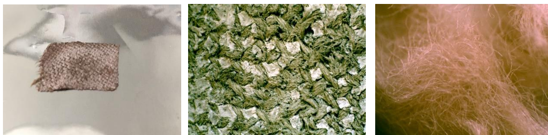
Fig. 2. RoAMS 297.60 („Rembrandt”) sample at various stages of the pretreatment: beginning of the chemical treatment (left); after Soxhlet treatment (center); pure canvas fiber obtained at the end, after ABA treatment (right).
