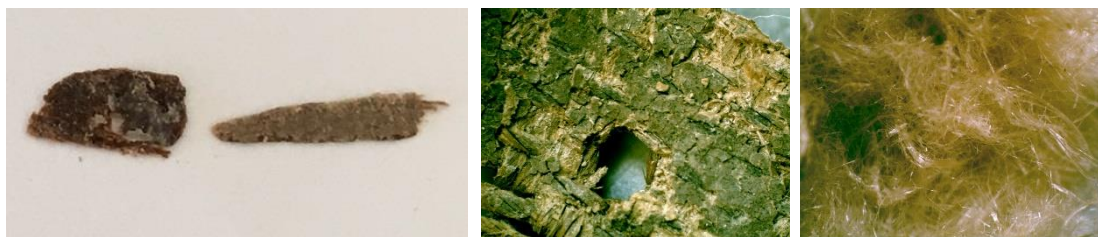
Fig.1. RoAMS 298.60 „Modigliani” sample, at the beginning (left), after Soxhlet treatment (center) and ABA treatment (right). Brown primer layer covering the vegetal fiber of the canvas is observed at the beginning of the treatment while at the end the vegetal fibers are completely cleaned.
