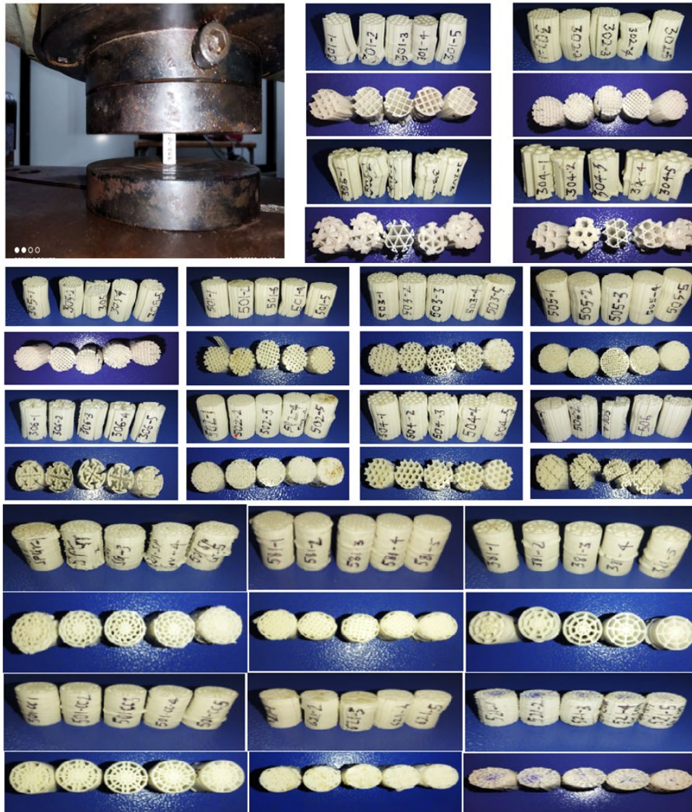
Fig. 7: Compression testing of all samples as per ASTM D695 standard
