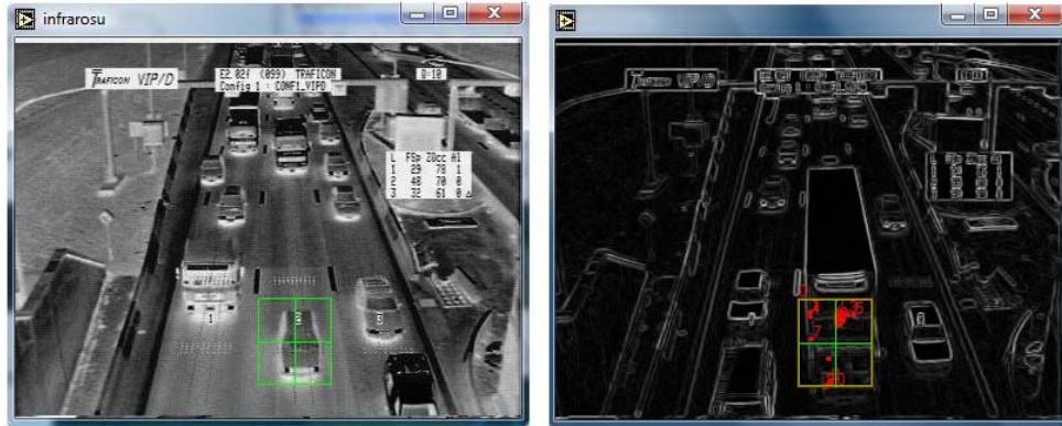
Fig. 6. The video stream before (left) and after (right) processing.
