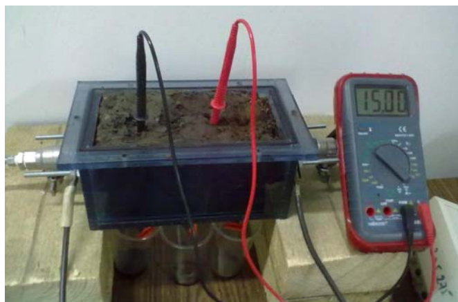
Fig.1. The experimental setup IPER 1 – electrochemical cell and the multimeter
