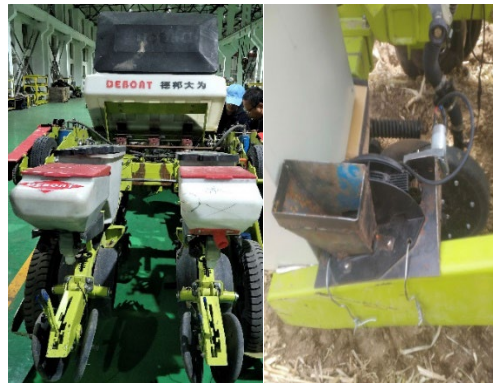
a: Photo of the planter, b: Seeding experiment Fig. 11 Electrically driven seed dischargers tester
