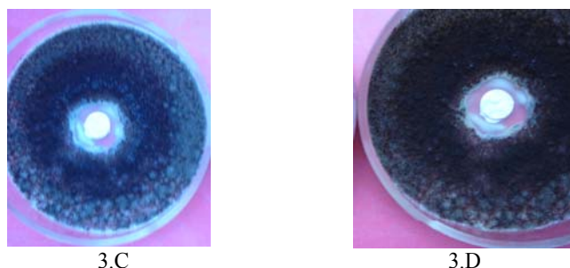
Fig. 3. The antifungal effect of antimicrobial coating materials: 3.A - antifungal effect of MPAS at 3 days; 3.B - antifungal effect of MP 9, at 3 days; 3.C - antifungal effect of MP 9, at 14 days; 3.D - antifungal effect of MP 9, at 28 days
