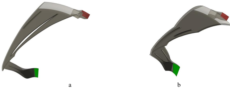
Fig. 2 Computational domain, initial compressor stage (a) and optimized compressor stage (b)
