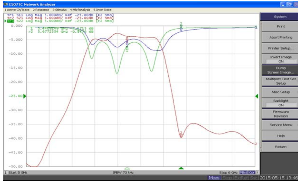
Fig.11 the measured characteristics of the filter
