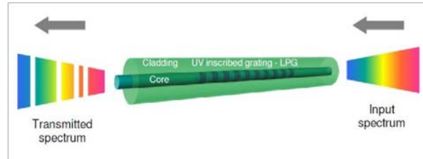
Fig. 1. Schematic representation of a LPGFS and its operation mode [12].
