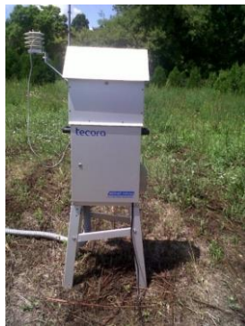
Fig. 3. High Volume Sampler (HVS) for the ambient air TSP identification
