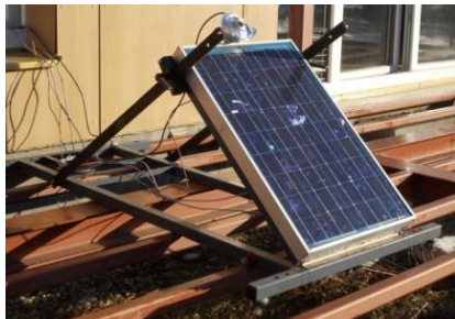
Fig. 1. BP Solar SX40U connected to Keithley data logger
