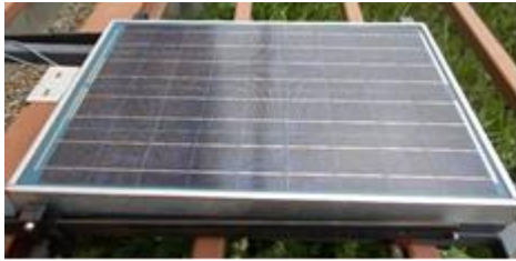
Fig. 7. Photovoltaic panel covered by 1,72g during 2 weeks in summer
