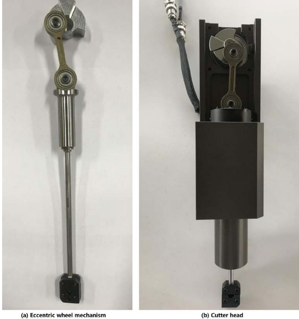
Fig.9. New mechanism of eccentric wheel and the complete cutting head
