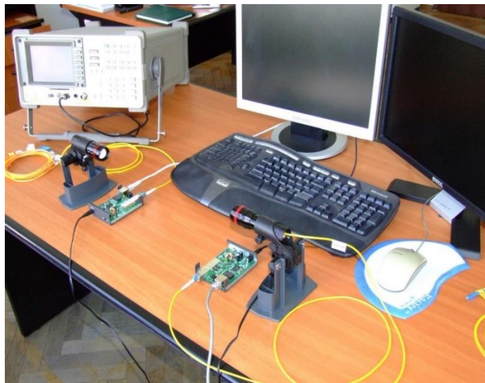
Fig. 5. WDM - FSO Laboratory Experimental Device – Component disposal
