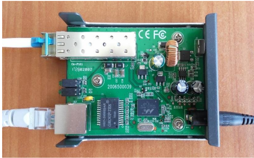
Fig. 6. Experimental laboratory device WDM - FSO - media-converter [12]
