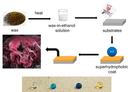
Fig. 1. Schematic illustration of the procedure for solution preparation and coating treatment
