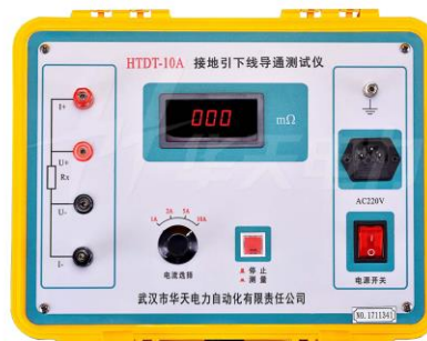
(a) The multi-channel corrosion detection system (b) The earth continuity tester Fig.4 The designed system and the earth continuity tester.
