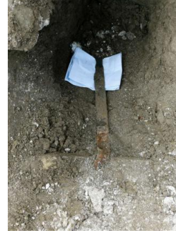
(a) Excavation result of No. 65 down conductor (b) Excavation result of nodes 90-100
