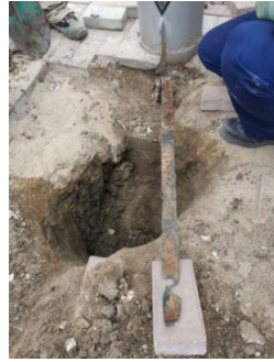
(a) Excavation result of No. 65 down conductor (b) Excavation result of nodes 90-100
