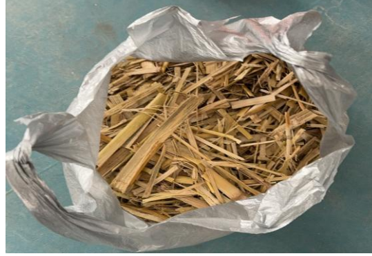
Fig. 1. Corn stalks after removal of core and pith
