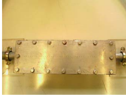
Fig. 5. The FBG assembly: FBG body and the plate fastened with screws.
