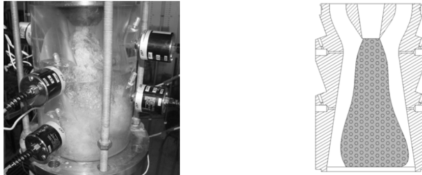
Fig. 6. Photo of the cavitating vortex rope on test rig with air admission at tank pressures of 0.2 bar (left) and its schematic representation (right).
