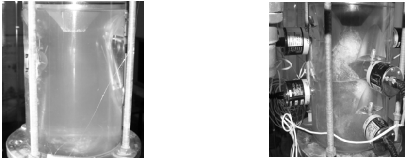
Fig. 5. Photos of non-cavitating (left) and cavitating (right) vortex ropes, respectively on test rig.
