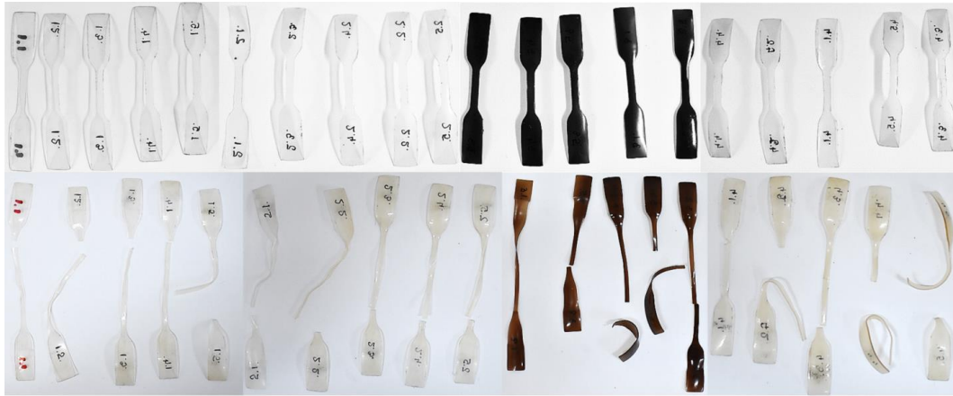
Fig. 5. Sample appearance before and after tensile testing
