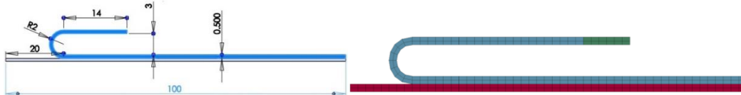
Fig. 4. Physical and discretization model of peeling test specimens
