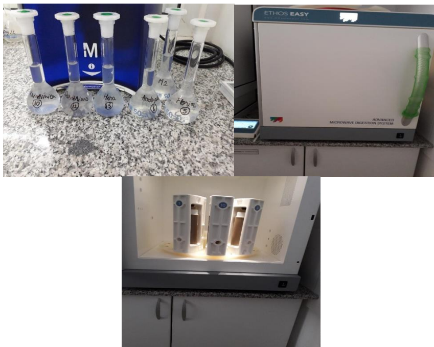
Fig. 3. Images of the samples subjected to digestion by ETHOS UP microwaves.
