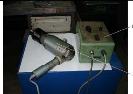
Fig. 2. Tapping device for electroerosion of machine CHARMILLES D4.
