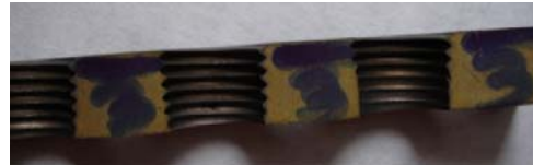
Fig. 4. Thread M12,5x1,5 machined in sinterised metallic carbide G20
