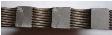
Fig. 3. Thread M12,5x1,5 machined in steel OLC45
