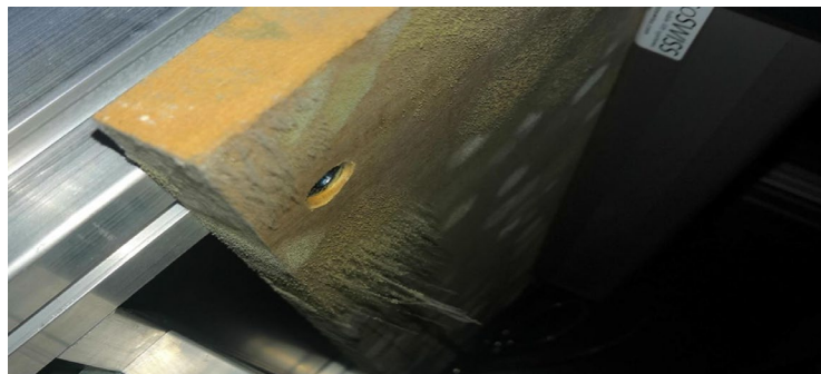
Fig. 9 - Mold stains on the inside of the Prosorb compartment in showcases exposed for a long time to an RH beyond the limits of preservation
