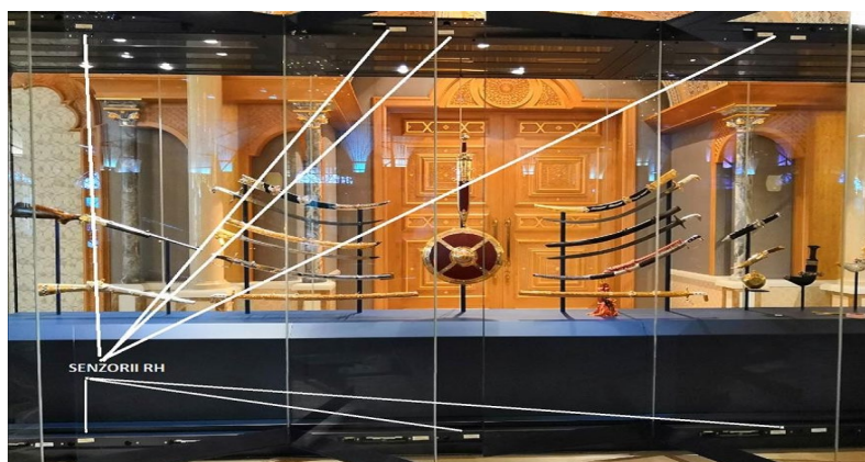
Fig. 7 – Humidity/temperature sensors placed under the base of the display case next to the Prosorb boxes and at the top. The interior height of the window is 2.6 meters.
