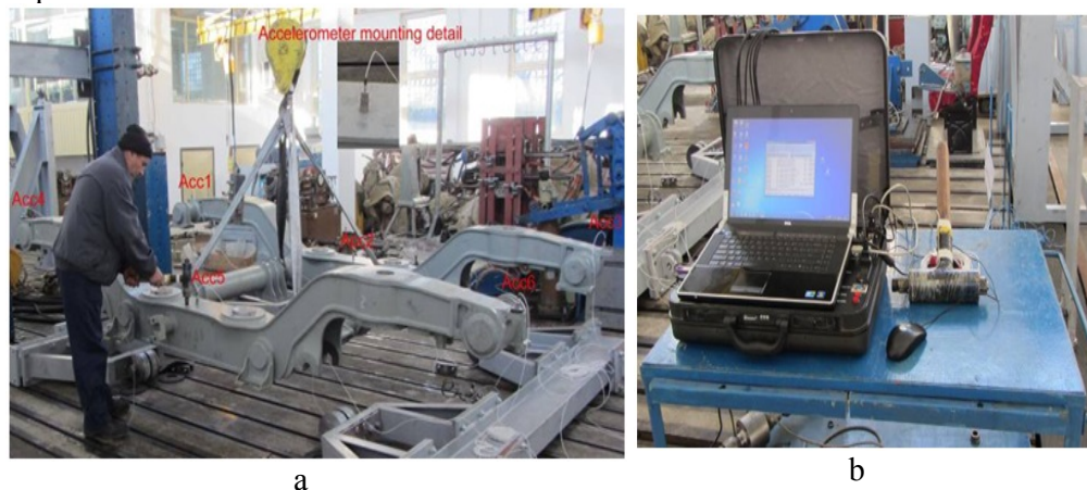
Fig.5 Experiments for modal identification of a bogie frame. a- Accelerometers locations. b- The impact hammer.
