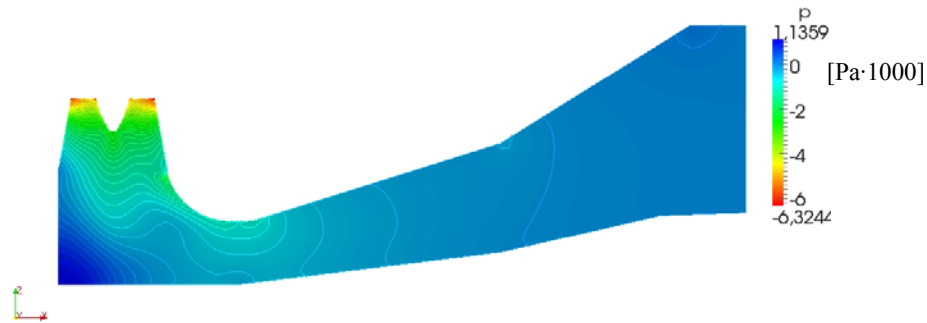
Fig. 10 Pressure variation between section 1 and the end the draft tube
