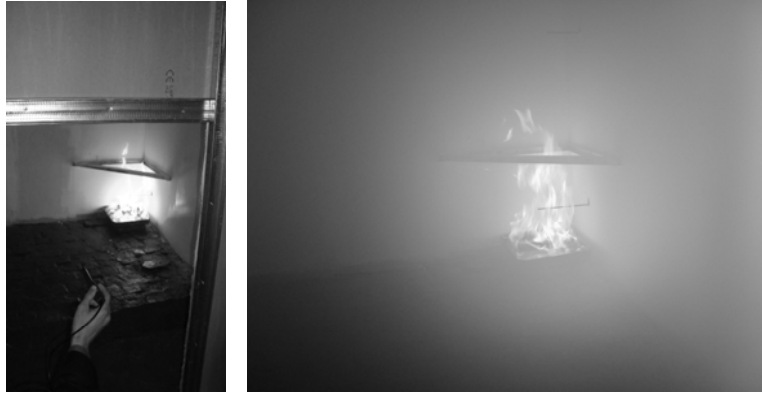
Fig. 4. Images taken during tests. From left to right: Ethanol pan fire before the water mist discharge, and during the water mist discharge
