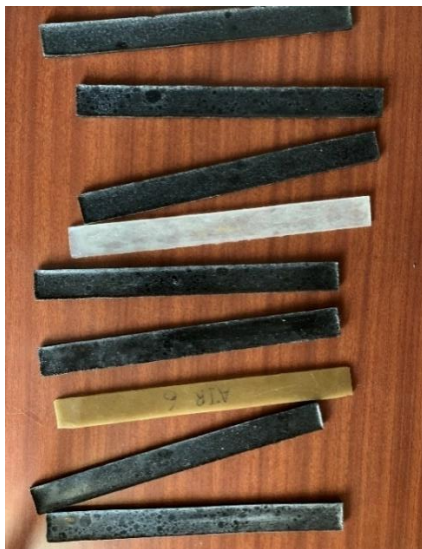
Fig. 1. Tensile samples prepared according to ASTM D3039
