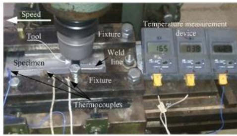
Fig. 2. Temperature measurements during friction stir welding process
