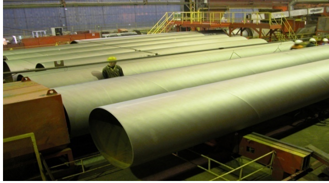
Fig. 2 Rolled pipes being prepared for the technical quality control process (QCP)
