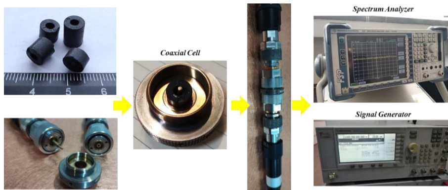
Fig. 1. Electromagnetic shielding measurements setup
