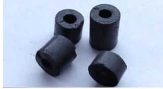
Fig. 3. High entropy alloys metallic powder compacted into ring shape samples
