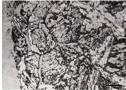
Fig. 11. Optical micrograph of the diffusion zone for sample E2. Reagent: Nital 2%.
