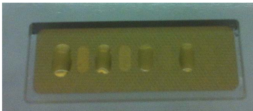
Fig. 1 Photographic image of glass prism with individual measuring channels and hydroxyapatite deposition
