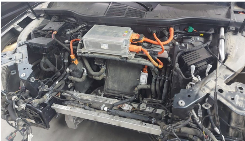
Fig. 23. Front space of the tested full electric car (free of front engine hood for inspection)
