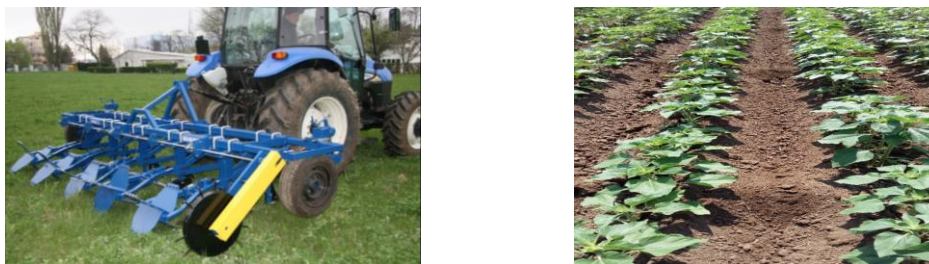
Fig.2. Device for soil modeling in interrupted furrows DMBC5-0 and the form of the furrows it made, [1]
