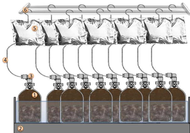
Fig. 1. Experimental set-up: (1) glass serum bottles; (2) thermostatic water bath; (3) connection system; (4) connection tube; (5) gas collecting bag; (6) hanging system for gas bags.
